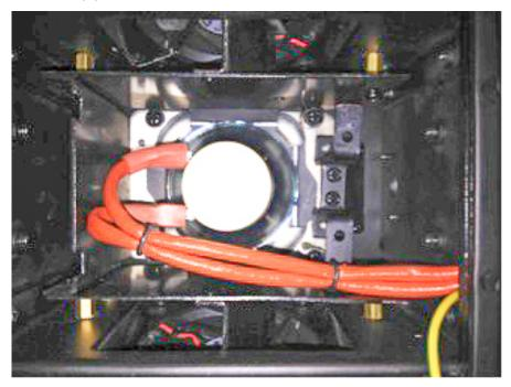
10. Replace the lamp cover back into place by securing (4) screws marked "A", "B", "C", and "D".
