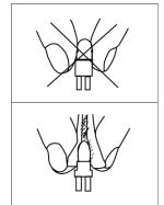
This fixture is fitted with a DISCHARGE LAMP, which is highly susceptible to damage if improperly handled. NEVER touch the lamp with your bare hands, as the oil from your hands will shorten the life of the lamp. Also, NEVER move the fixture until the lamp has had ample time to cool. Lamps are NOT covered under warranty conditions.
