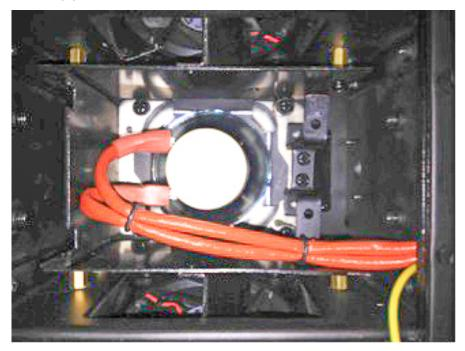
3. Using two fingers on your **RIGHT** hand, pull the retention handle **OUT** and towards the **RIGHT** as far as possible.
