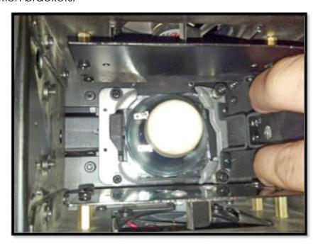
8. Release the retention handle with your **RIGHT** hand and make sure the handle is upright and not at an angle.
