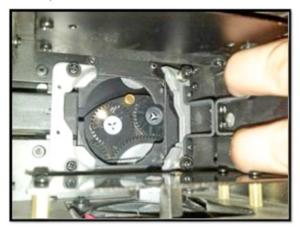
6. While pulling the retention handle with your **RIGHT** hand, use your **LEFT** had to gently install the lamp under the retention brackets by holding the lamp at a slight angle and positioning it until it is flush with the base.
